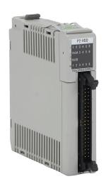
Productivity2000 pulse output module, 1 MHz maximum switching frequency, 4 high-speed output point(s), 5-24 VDC, sinking/sourcing, 2-channel, differential and single-ended output channel(s), 6 high-speed input point(s), 5-24 VDC, sinking/sourcing, external 24 VDC required.
