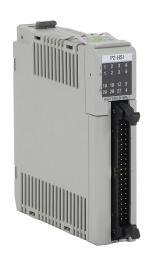
Productivity2000 pulse input module, 1 MHz maximum switching frequency, 2 high-speed input point(s), 5-24 VDC, sinking/sourcing, 2-channel, differential and single-ended encoder input(s), 4 high-speed output point(s), 5-24 VDC, sinking/sourcing, external 24 VDC required.
