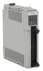
Productivity2000 pulse input module, 1 MHz maximum switching frequency, 2 high-speed input point(s), 5-24 VDC, sinking/ sourcing, 2-channel, differential and single-ended encoder input(s), 4 high-speed output point(s), 5-24 VDC, sinking/ sourcing, external 24 VDC required.
