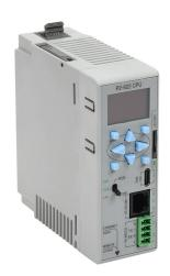
Productivity2000 CPU, up to 50 MB ladder memory, 4 x 10 character OLED display, microSD card slot, (2) Ethernet 10/100Base-T (RJ45), (1) RS-232/RS-485 (RJ12), (1) RS-232/RS-485 (4-pin terminal) and (1) USB C port(s), battery included.
