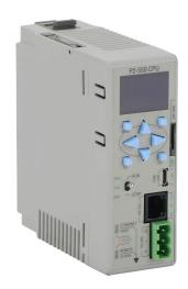
Productivity2000 CPU, up to 50 MB ladder memory, 4 x 10 character OLED display, microSD card slot, (2) Ethernet 10/100Base-T (RJ45), (1) RS-232 (RJ12), (1) RS-485 (3-pin terminal) and (1) microB-USB port(s), battery included.
