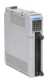
Productivity2000 discrete input module, 32-point, 24 VAC/VDC, sinking/sourcing, 4 isolated common(s), 8 point(s) per common. Requires ZIPLink connector modules and pre-wired cables.
