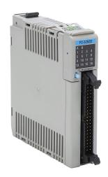
Productivity2000 discrete input module, 32-point, 12-24 VDC, sinking/sourcing, 4 isolated common(s), 8 point(s) per common. Requires ZIPLink connector modules and pre-wired cables.
