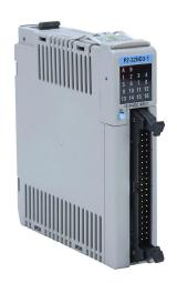
Productivity2000 discrete input module, 32-point, 12-24 VDC, sinking/sourcing, 4 isolated common(s), 8 point(s) per common. Requires ZIPLink connector modules and pre-wired cables.
