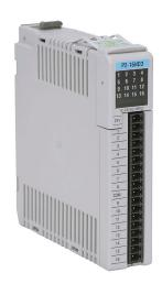
Productivity2000 discrete input module, 16-point, 12-24 VDC, sinking/sourcing, 1 isolated common(s), 16 point(s) per common. Requires P2-RTB or P2-RTB-1 removable terminal block or ZIPLink pre-wired cables.
