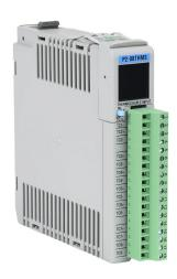
Productivity2000 temperature input module, thermocouple, 8-channel, 16-bit resolution, isolated, input thermocouple type(s): J, E, K, R, S, T, B, N, C. (1) P2-RTB screw terminal block included.
