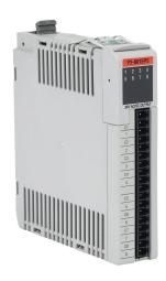
Productivity2000 relay output module, 8-point, 24 VAC/VDC, (8) solid state relays, 8 isolated common(s), 1 point(s) per common, 1A/point @ 50 °C, 0.75A/point @ 60 °C. Requires P2-RTB or P2-RTB-1 removable terminal block or ZIPLink pre-wired cables.
