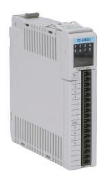
Productivity2000 discrete input module, 8-point, 12-24 VDC, sinking/sourcing, 1 isolated common(s), 8 point(s) per common. Requires P2-RTB or P2-RTB-1 removable terminal block or ZIPLink pre-wired cables.
