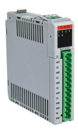
Productivity2000 relay output module, 6-point, 5-30 VDC/5-264 VAC, (5) Form A, (1) Form C, 6 isolated common(s), 1 point(s) per common, 7A/point. Requires P2-RTB13 or P2-RTB13-1 removable terminal block.
