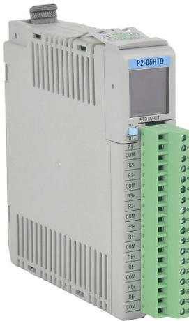
Productivity2000 temperature input module, RTD, 6-channel, 16-bit resolution, input RTD type(s): Pt100, Pt1000, JPt100, Cu10, Cu25 and Ni120. (1) P2-RTB screw terminal block included.
