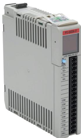
Productivity2000 analog output module, 4-channel, voltage, 16-bit, output voltage signal range(s) of +/- 10 VDC, external 24 VDC required.
