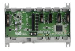
Productivity2000 I/O base, 4-slot, DIN rail or flush mount. Requires P2-01AC, P2-01DCAC or P2-01DC power supply. Holds power supply, CPU and (4) I/O modules.
