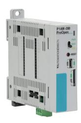
ProductivityOpen Arduino-compatible CPU, CircuitPython and C++, microSD card slot, (1) microB-USB port(s), external 24 VDC required. For use with ProductivityOpen shields, Arduino MKR series shields and Productivity1000 expansion modules.
