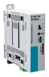
ProductivityOpen Arduino-compatible CPU, C++, microSD card slot, (1) microB-USB port(s), external 24 VDC required. For use with ProductivityOpen shields, Arduino MKR series shields and Productivity1000 expansion modules.
