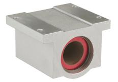
PBC Simplicity series single pillow block, plain bearing, 2.81in overall length, PTFE, 1in inside diameter, aluminum housing, 0.0015in running clearance. For use with 1in diameter PBC shafts.
