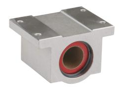
PBC Simplicity series single pillow block, plain bearing, 2.06in overall length, PTFE, 3/4in inside diameter, aluminum housing, 0.0005in running clearance. For use with 3/4in diameter PBC shafts.
