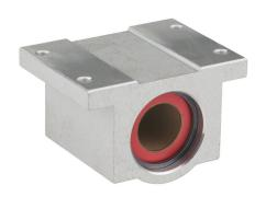
PBC Simplicity series single pillow block, plain bearing, 2.06in overall length, PTFE, 3/4in inside diameter, aluminum housing, 0.0015in running clearance. For use with 3/4in diameter PBC shafts.
