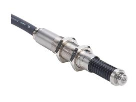
Metrol limit switch, high precision touch, 10mm diameter, threaded, 0.5mm pitch, 70mm length, 2mm round head, stainless steel, 8.5mm plunger, 1N contact force, N.C. contact(s), 9.8ft/3m cable length, pigtail.
