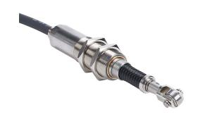
Metrol limit switch, high precision touch, 14mm diameter, threaded, 0.5mm pitch, 84.5mm length, 8mm roller head, stainless steel, 2.5mm plunger, 1N contact force, (1) N.C. contact(s), 9.8ft/3m cable length, pigtail.
