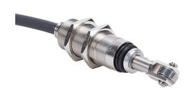
Metrol limit switch, high precision touch, 14mm diameter, threaded, 0.5mm pitch, 55mm length, 8mm roller head, stainless steel, 2.5mm plunger, 1N contact force, (1) N.C. contact(s), 9.8ft/3m cable length, pigtail.
