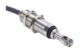
Metrol limit switch, high precision touch, 14mm diameter, threaded, 0.5mm pitch, 61mm length, 8mm roller head, stainless steel, 2.5mm plunger, 1N contact force, (1) N.O. contact(s), 9.8ft/3m cable length, pigtail.
