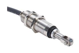
Metrol limit switch, high precision touch, 14mm diameter, threaded, 0.5mm pitch, 61mm length, 8mm roller head, stainless steel, 2.5mm plunger, 1N contact force, N.O. contact(s), 9.8ft/3m cable length, pigtail.
