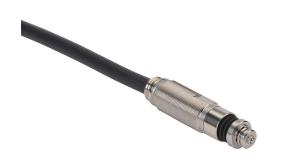
Metrol limit switch, high precision touch, 10mm diameter, threaded, 0.5mm pitch, 42mm length, 2mm round head, stainless steel, 8.5mm plunger, 1N contact force, (1) N.C. contact(s), 9.8ft/3m cable length, pigtail.
