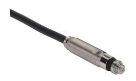
Metrol limit switch, high precision touch, 10mm diameter, threaded, 0.5mm pitch, 49.8mm length, 2mm round head, stainless steel, 8.5mm plunger, 1N contact force, (1) N.O. contact(s), 9.8ft/3m cable length, pigtail.
