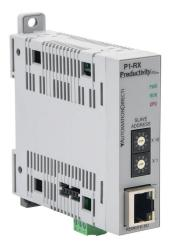
Productivity1000 remote I/O module, 1 port, (1) Ethernet (RJ45) port(s). For use with P1-550, P2-550 and P2-622 CPUs.
