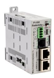
Productivity1000 CPU, up to 50 MB ladder memory, microSD card slot, (2) Ethernet 10/100Base-T (RJ45), (1) RS-232 (RJ12), (1) RS-485 (4-pin terminal) and (1) microB-USB port(s), external 24 VDC required, battery included.
