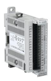
Productivity1000 discrete combo module, Input: 8-point, 24 VAC/ VDC, sinking/sourcing, Output: 4-point, 6–30 VDC / 6–120 VAC, relay, (4) Form A (SPST) relays, 5A/point, 2A/point if used with ZIPLink cable.
