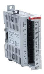
Productivity1000 relay output module, 8-point, 6-24 VDC/6-120 VAC, (6) Form A, (2) Form C, 8 isolated common(s), 1 point(s) per common, 3A/point. Requires P2-RTB or P2-RTB-1 removable terminal block or ZIPLink pre-wired cables.
