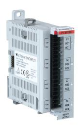
Productivity1000 relay output module, 4-point, 5-30 VDC/5-264 VAC, (4) Form C, 4 isolated common(s), 1 point(s) per common, 7A/point. Requires P2-RTB or P2-RTB-1 removable terminal block.
