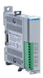
Productivity1000 temperature input module, thermocouple, 4-channel, 16-bit resolution, input thermocouple type(s): J, E, K, R, S, T, B, N, C. (1) P1-10RTB screw terminal block included.
