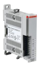
Productivity1000 relay output module, 4-point, 24 VAC/VDC, (4) solid state relays, 4 isolated common(s), 1 point(s) per common, 1A/point @ 50 °C, 0.75A/point @ 60 °C. Requires P1-10RTB or P1-10RTB-1 removable terminal block or ZIPLink pre-wired cables.
