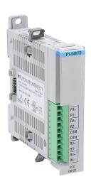
Productivity1000 temperature input module, RTD, 4-channel, 16-bit resolution, input RTD type(s): Pt100, Pt1000, JPt100, Cu10, Cu25 and Ni120. (1) P1-10RTB screw terminal block included.
