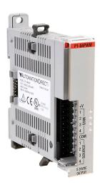
Productivity1000 high-speed pulse width modulation output module, 5-24 VDC, sinking/sourcing, 4-channel, single-ended output(s), external 5-24 VDC required.
