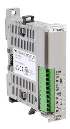
Productivity1000 counter input module, 100 kHz maximum switching frequency, 2 high-speed input point(s), 5-24 VDC, sinking/sourcing, 2-channel, single-ended encoder input(s), external 24 VDC required.
