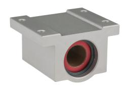
PBC Simplicity series single pillow block, plain bearing, 1.69in overall length, PTFE, 1/2in inside diameter, aluminum housing, 0.0005in running clearance. For use with 1/2in diameter PBC shafts.
