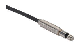
Metrol limit switch, high precision touch, 8mm diameter, threaded, 0.5mm pitch, 48.8mm length, 2mm round head, stainless steel, 5.5mm plunger, 1N contact force, N.C. contact(s), 9.8ft/3m cable length, pigtail.
