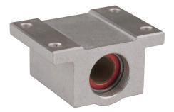
PBC Simplicity series single pillow block, plain bearing, 1.31in overall length, PTFE, 3/8in inside diameter, aluminum housing, 0.0005in running clearance. For use with 3/8in diameter PBC shafts.
