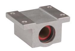
PBC Simplicity series single pillow block, plain bearing, 1.31in overall length, PTFE, 3/8in inside diameter, aluminum housing, 0.0015in running clearance. For use with 3/8in diameter PBC shafts.
