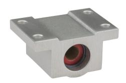
PBC Simplicity series single pillow block, plain bearing, 1.19in overall length, PTFE, 1/4in inside diameter, aluminum housing, 0.0005in running clearance. For use with 1/4in diameter PBC shafts.
