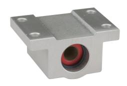
PBC Simplicity series single pillow block, plain bearing, 1.19in overall length, PTFE, 1/4in inside diameter, aluminum housing, 0.0015in running clearance. For use with 1/4in diameter PBC shafts.
