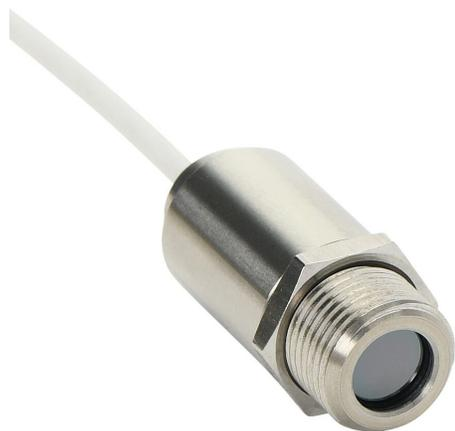
Optris CSmicro LTH infrared pyrometer, -50 to 1030 deg C, 8-14  $\mu\text{m}$  spectral range, 0-5 VDC, 0-10 VDC, alarm or pulse output, 5-30 VDC operating voltage, M12x1 threaded end mount, 6m integral 5-conductor shielded cable.
