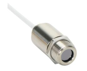
Optris CSmicro LTH infrared pyrometer, -50 to 1030 deg C, 8-14 µm spectral range, 0-5 VDC, 0-10 VDC, alarm or pulse output, 5-30 VDC operating voltage, M12x1 threaded end mount, 1m integral 5-conductor shielded cable.
