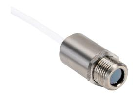
Optris CSmicro LT infrared pyrometer, -50 to 1030 deg C, 8-14  $\mu$ m spectral range, 0-5 VDC, 0-10 VDC, alarm or pulse output, 5-30 VDC operating voltage, M12x1 threaded end mount, 6m integral 5-conductor shielded cable.
