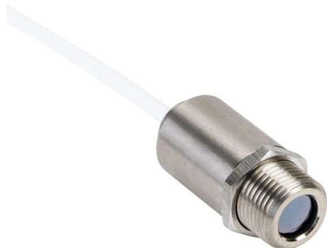
Optris CSmicro LT infrared pyrometer, -50 to 1030 deg C, 8-14  $\mu\text{m}$  spectral range, 0-5 VDC, 0-10 VDC, alarm or pulse output, 5-30 VDC operating voltage, M12x1 threaded end mount, 1m integral 5-conductor shielded cable.
