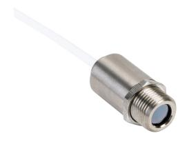
Optris CSmicro LT infrared pyrometer, -50 to 1030 deg C, 8-14  $\mu$ m spectral range, 0-5 VDC, 0-10 VDC, alarm or pulse output, 5-30 VDC operating voltage, M12x1 threaded end mount, 1m integral 5-conductor shielded cable.
