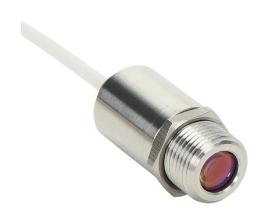
Optris CSmicro 3M infrared pyrometer, 50 to 350 deg C, 2.3  $\mu$ m spectral range, 0-5 VDC, 0-10 VDC, alarm or pulse output, 5-30 VDC operating voltage, M12x1 threaded end mount, 6m integral 5-conductor shielded cable.
