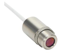
Optris CSmicro 3M infrared pyrometer, 50 to 350 deg C, 2.3 µm spectral range, 0-5 VDC, 0-10 VDC, alarm or pulse output, 5-30 VDC operating voltage, M12x1 threaded end mount, 1m integral 5-conductor shielded cable.
