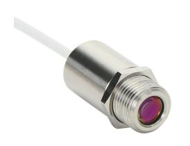
Optris CSmicro 3M infrared pyrometer, 100 to 600 deg C, 2.3 µm spectral range, 0-5 VDC, 0-10 VDC, alarm or pulse output, 5-30 VDC operating voltage, M12x1 threaded end mount, 6m integral 5-conductor shielded cable.
