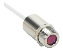
Optris CSmicro 3M infrared pyrometer, 100 to 600 deg C, 2.3  $\mu m$  spectral range, 0-5 VDC, 0-10 VDC, alarm or pulse output, 5-30 VDC operating voltage, M12x1 threaded end mount, 1m integral 5-conductor shielded cable.
